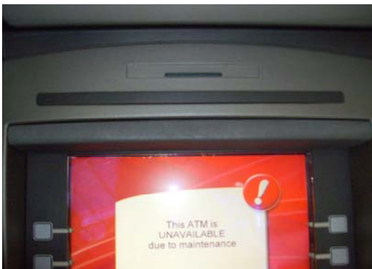
3. Close up of pinhole camera housing
