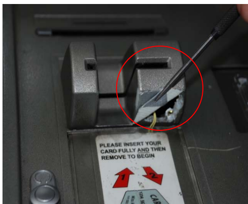
2. The damaged Card reader
