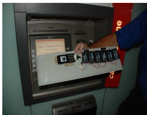
4. Mobile phone being used to capture PIN, which was concealed in the light cavity of the ATM
