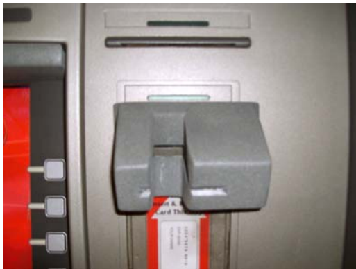
3. Close up of pinhole camera housing
