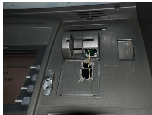
4. Mobile phone being used to capture PIN, which was concealed in the light cavity of the ATM
